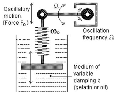
*Figure 1. Forced oscillations in a medium of variable damping. The driving oscillating force is  $F_0$  and it is oscillating with frequency  $\Omega$ .*
